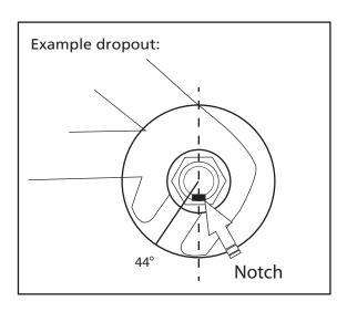
Cut out center hole, and place over axle.
